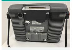
For maximum flexibility, Mentor UT can be configured with an industry standard Tyco or Ipex PA probe connector.
