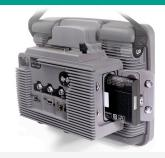
For maximum functionality, attach the MUX module and gain 32:128 capability, an additional hot swappable battery, and standard Tyco connector.
